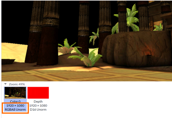
Figure 3-9: Format and data type of framebuffer attachments
